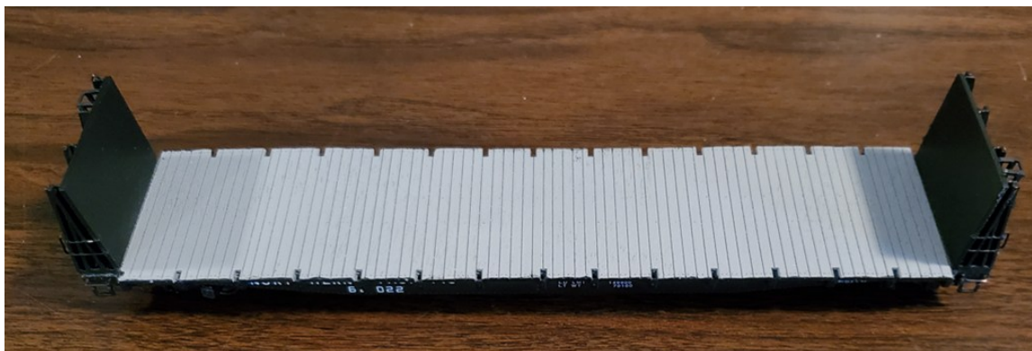
Sam Delauter's bulkhead flat car started as a regular flat car and received a new shorter deck that made room for the scratch built bulkheads. Ironically, the prototype did the same starting with a plain flat car!
